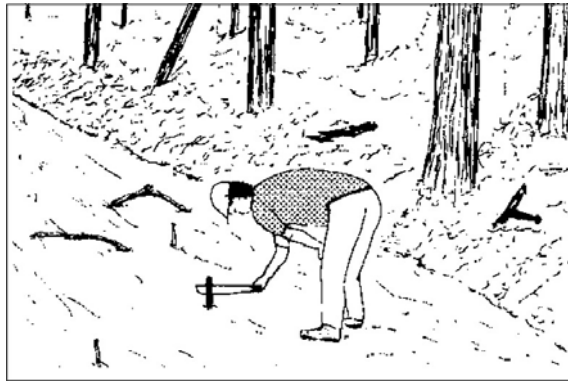
Figure 52 Remove stumps manually and not with the bulldozer so as not to disturb the topsoil, since this will lead to early rutting of trail and log market.
