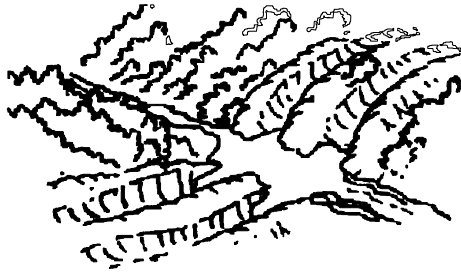
Skid trail crossing watercourse causing damage to stream banks and channel
