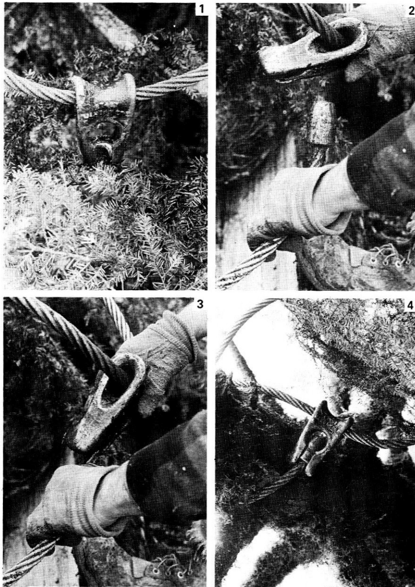
Setting a choker: (1) the Bardon or bell hook. (2) Choker setter has the ferrule in one hand and the bell in the other (3) the ferrule is placed in the bell and the cable is laid in the slot. (4) Choker is set and ready to go. The choker was placed over the log so that it will not become unhooked while the log is being skidded.
